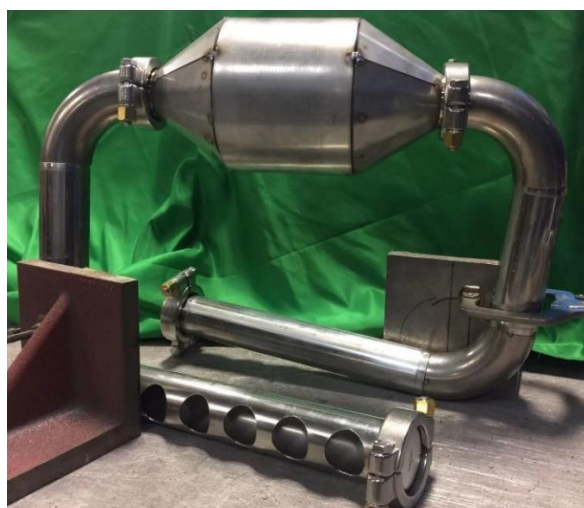
Fig. 2: The 2-L AGR assembly including accessory parts connected to the primary HXs in natural gas furnaces.
