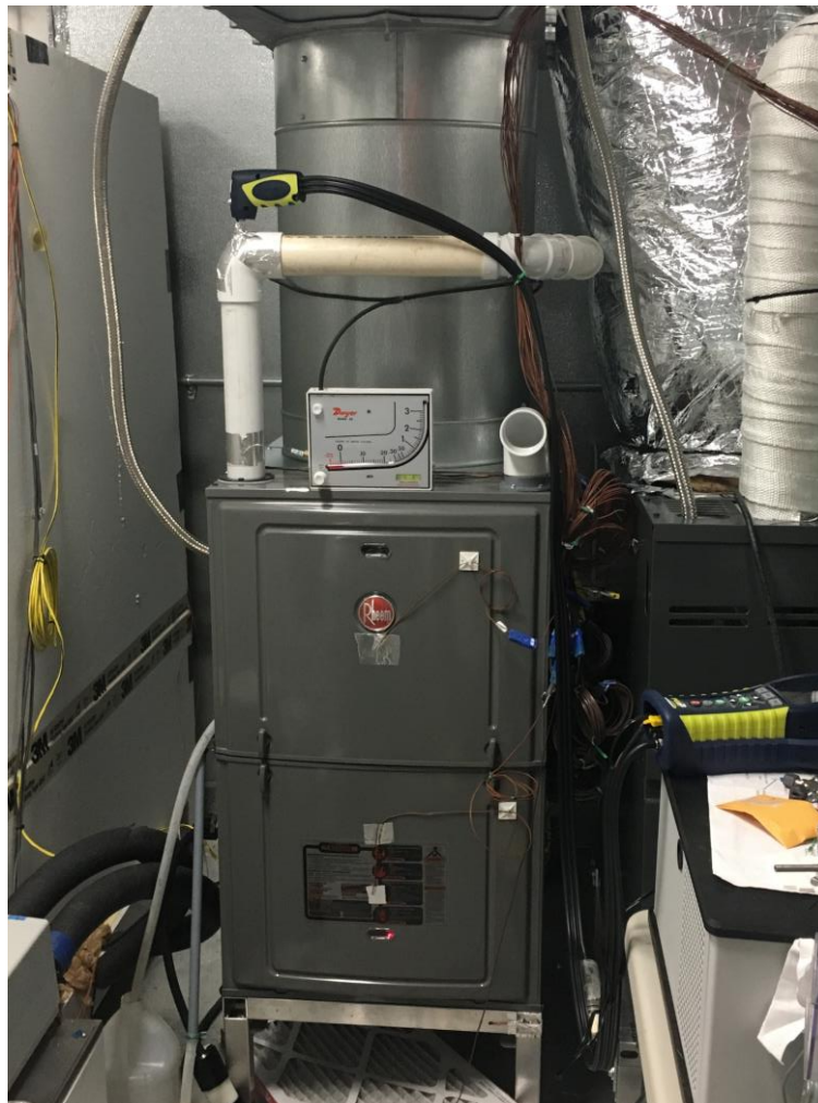
Fig. 4: The AGR-enabled 80 KBTU/h condensing furnace tested in a furnace testing chamber.
