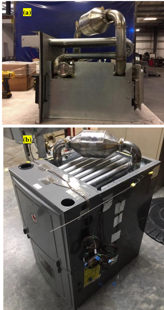
Fig. 3: (a) The integration of the fabricated AGR assembly with the primary HX of the Rheem condensing furnace; (b) the retrofitted furnace with AGR component.
